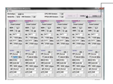
At the top part of the menu, the device data is displayed, such as type, serial number, hardware version and software versions for the CPU and FPGA.
