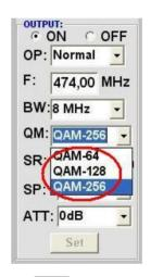
Settings of the possible QAM-Mode (16, 32, 64, 128, 256) are dependent on the data rate of the input transponder. Only the possible QAM- Mode will be displayed.
