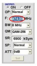
Frequency freely selectable It is recommended to keep the TV-Standard channel spacing. Eingestellt
