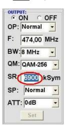
Up to 7.200 kiloSymbole/ sec. It is dependent on the selected QAM-Mode (usual setting in cable networks: 256 QAM / SR 6.900). Only the possible Symbol rates will be accepted.
