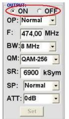
If not all 16 output channels are occupied, each channel can be individually turned off with **OFF**.
