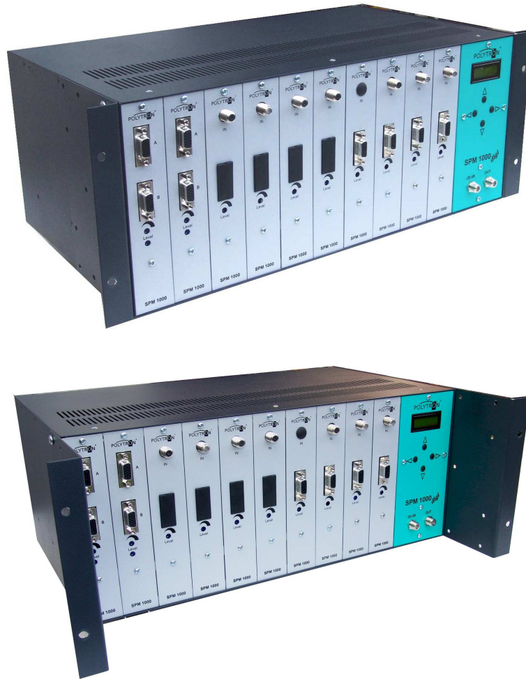
Figure 8 Installation in a 19" rack
