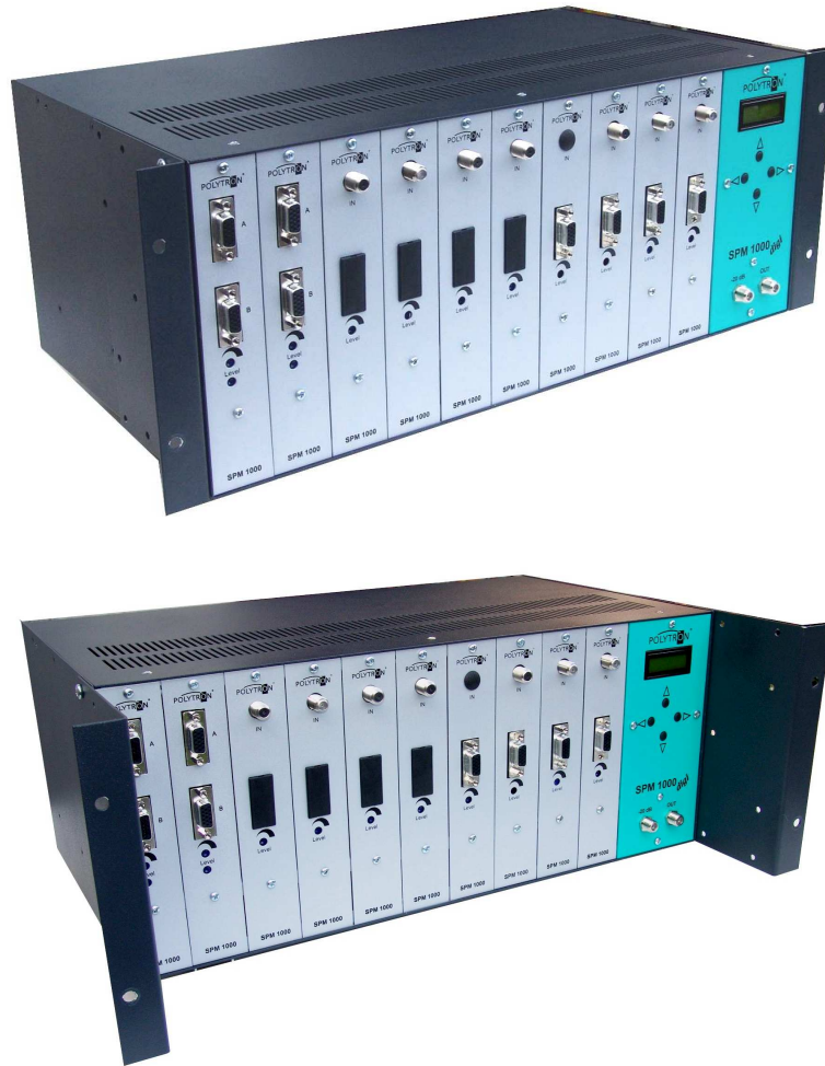
Figure 18 Installation in a 19" rack
